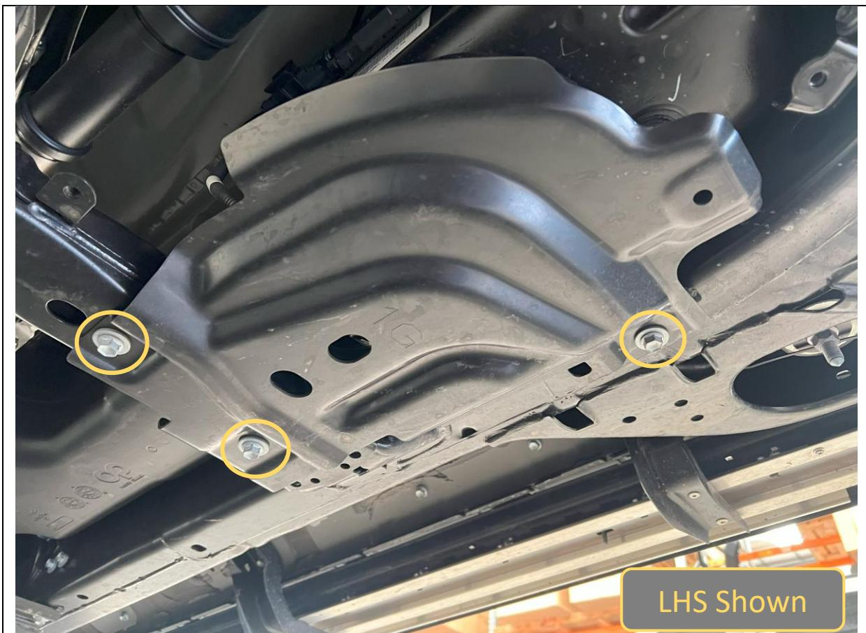
6. On the LHS of vehicle, remove the 3x 12mm Flange Head bolts securing the ad-blue tank guard to the chassis.
