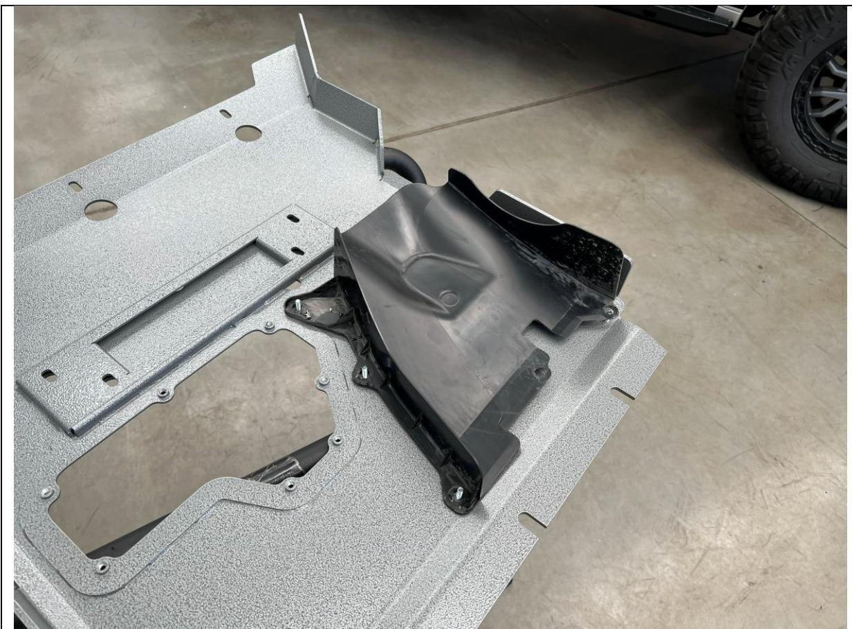
21. Fit the front differential air guide to the studs on the center bash plate assembly, using 6x M6 Flat washers and M6 Nyloc nuts.
