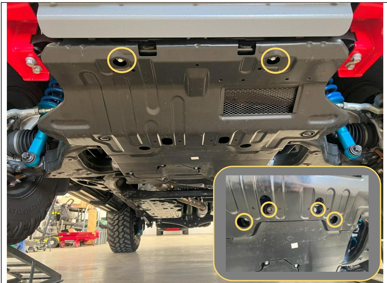
2. Remove factory forward splash shield panel, by removing the 6x 12mm head Flanged head hex bolts securing it to the chassis.
