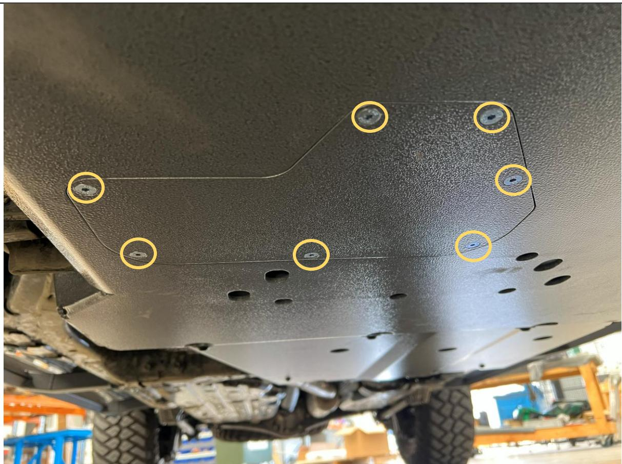
46. Fit the oil drain access cover plate using 7x M6x16 Countersunk screws into the captive nuts in the center bash plate assembly. Get all screws started before tightening.
