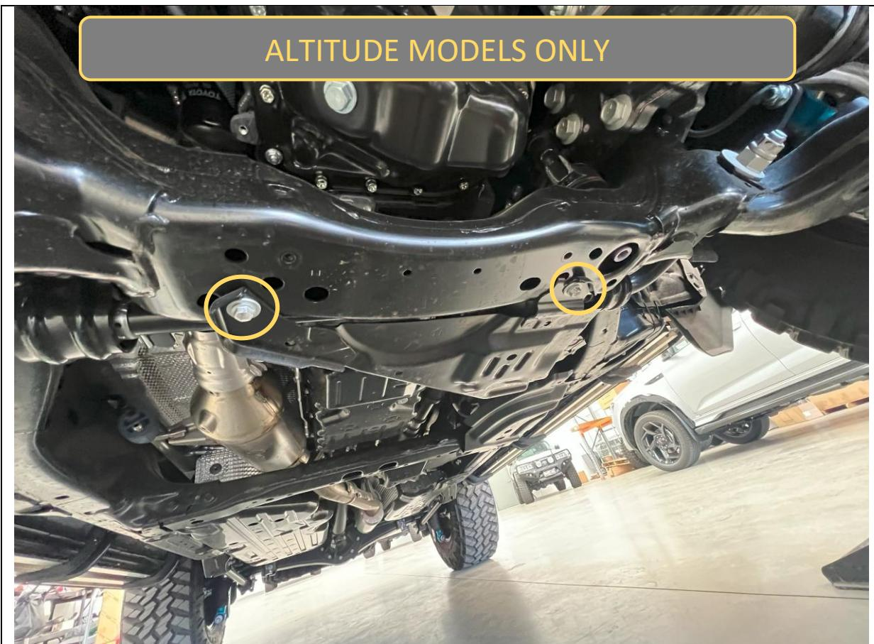
8. On Altitude models, remove the sway bar disconnect actuator guard, by removing the 2x 12mm head factory flange bolts that secure it to the chassis.
