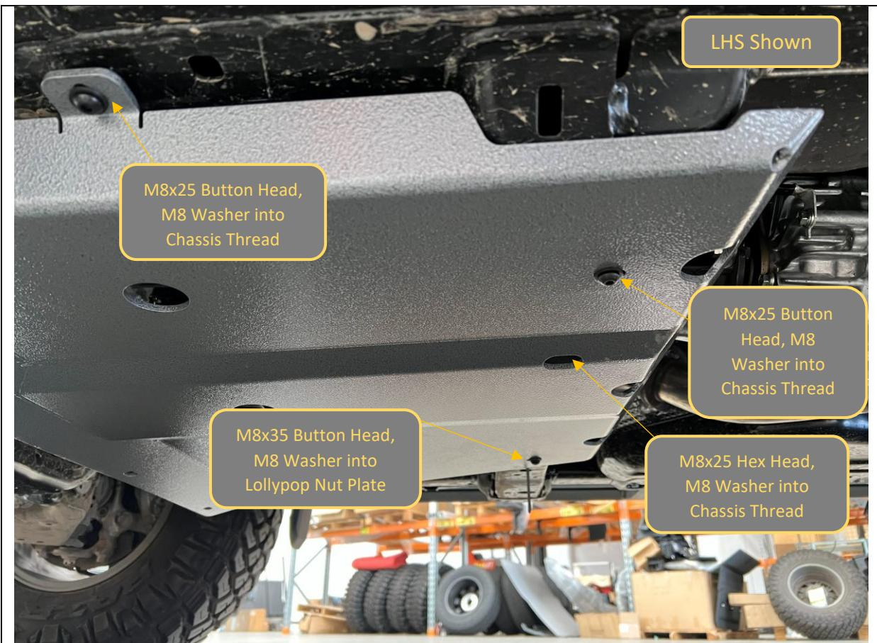
29. Fit the rear bash plate to the vehicle using the fasteners shown in the image.
